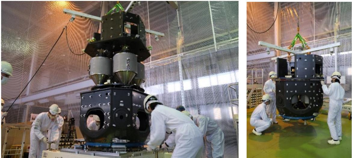
Photos of the structural thermal model of the HAKUTO-R M2 lunar lander being assembled at a Japan Airlines Facility in Narita Airport.
